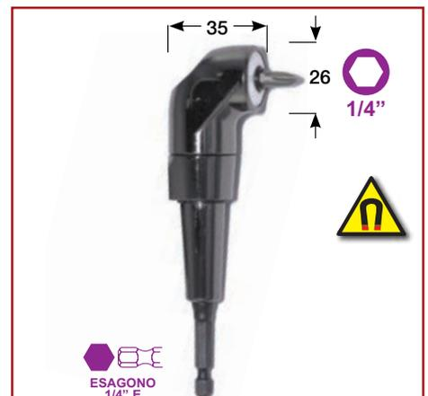
**PORTA INSERTI AD ANGOLO DI 90° - MAX 2000 GIRI AL MINUTO (RPM) - COPPIA MASSIMA 57 NM - IMPUGNATURA REGOLABILE**
